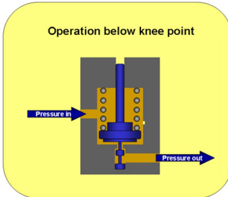
When the pressure in the circuit that the valve is connected to reaches a point where the resultant force exerted by the piston matches the spring preload, the piston lifts off of its seat and acts like an accumulator or a control valve as shown.
