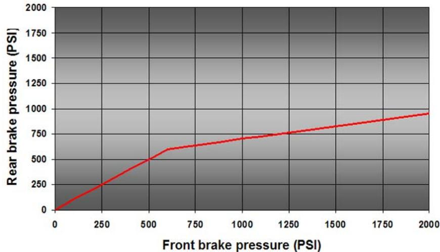
Due to the design of this valve, it should never be used on the front circuit because force output on the front should always directly respond to driver input without any limitation.
