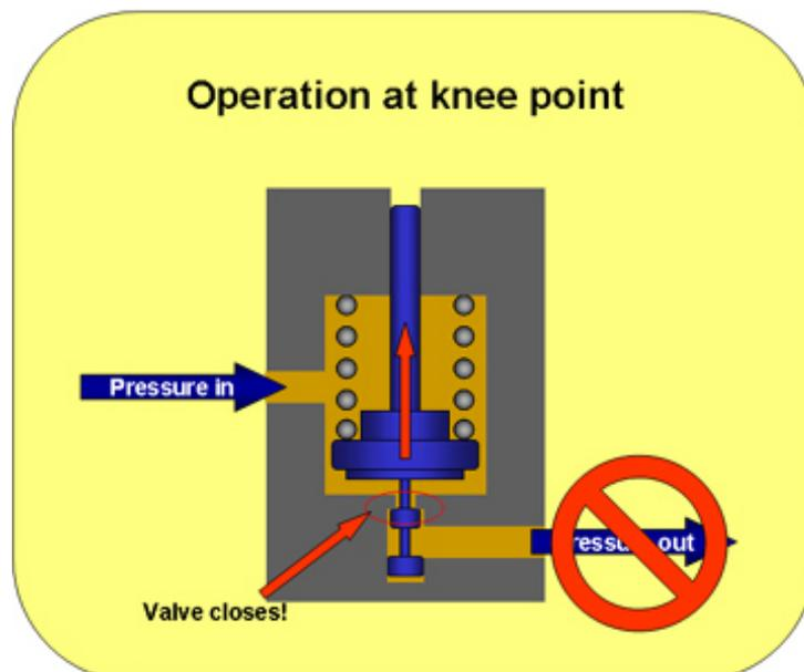
Any further increase in pressure is at a rate that equals the (relatively low) spring rate. On a graph showing pressure plotted against pedal force in the circuit that the valve is installed in, you will see a linear rise or slope up to the preset pressure (knee point) and then a sharp transition to a different slower rise rate or slope.
